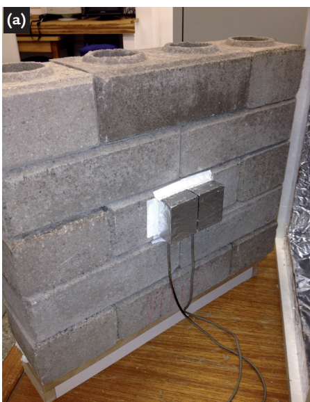
Figure 2 (a) Internal and (b) external temperature and heat flux sensor in the RCDW wall.
