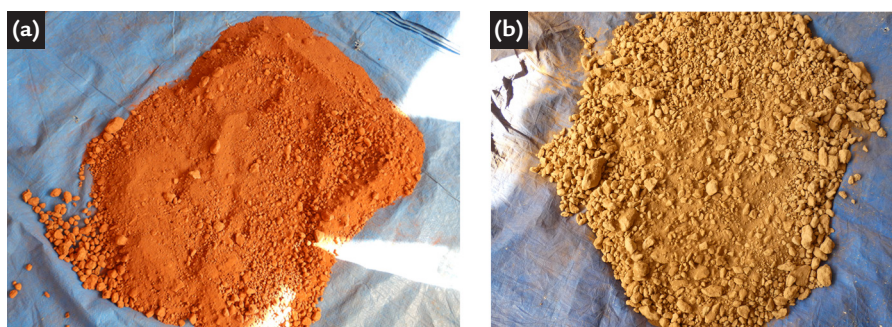
Figure 2 – a) Drying of Laterite LatJ2; (b) Drying of Laterite LatJ3.
