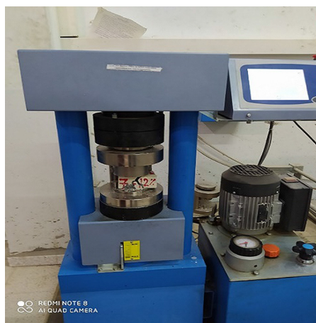
Figure 3 - Compressive strength test device of the \text{MDP}_{\text{Mix}} .
