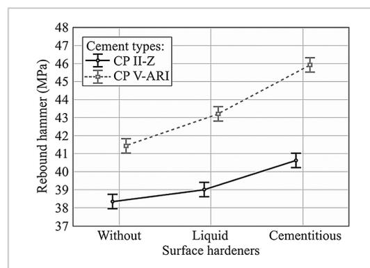
Figure 4 - Effects between the cement type and treatment type on the surface hardness.
