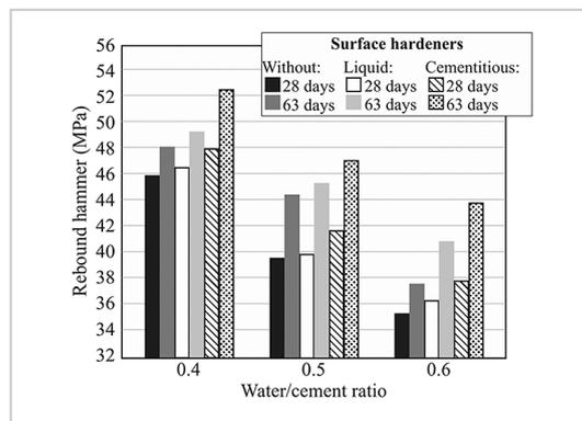
Figure 7 - Effects of interaction between the cement type, treatment type, and w/c ratios on surface hardness.
