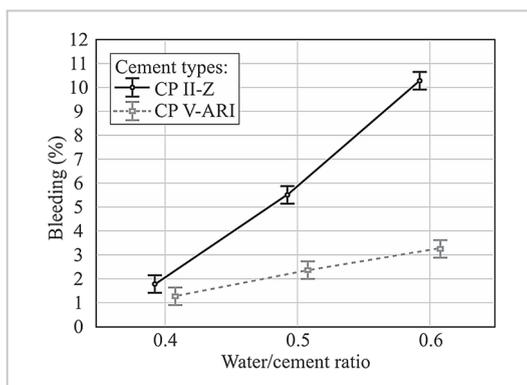
Figure 2 - Effects of interaction between the w/c ratio and cement type in the bleeding.
