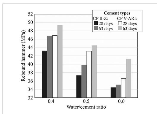
Figure 6 - Effects of cement type, age, and w/c ratio on surface hardness.
