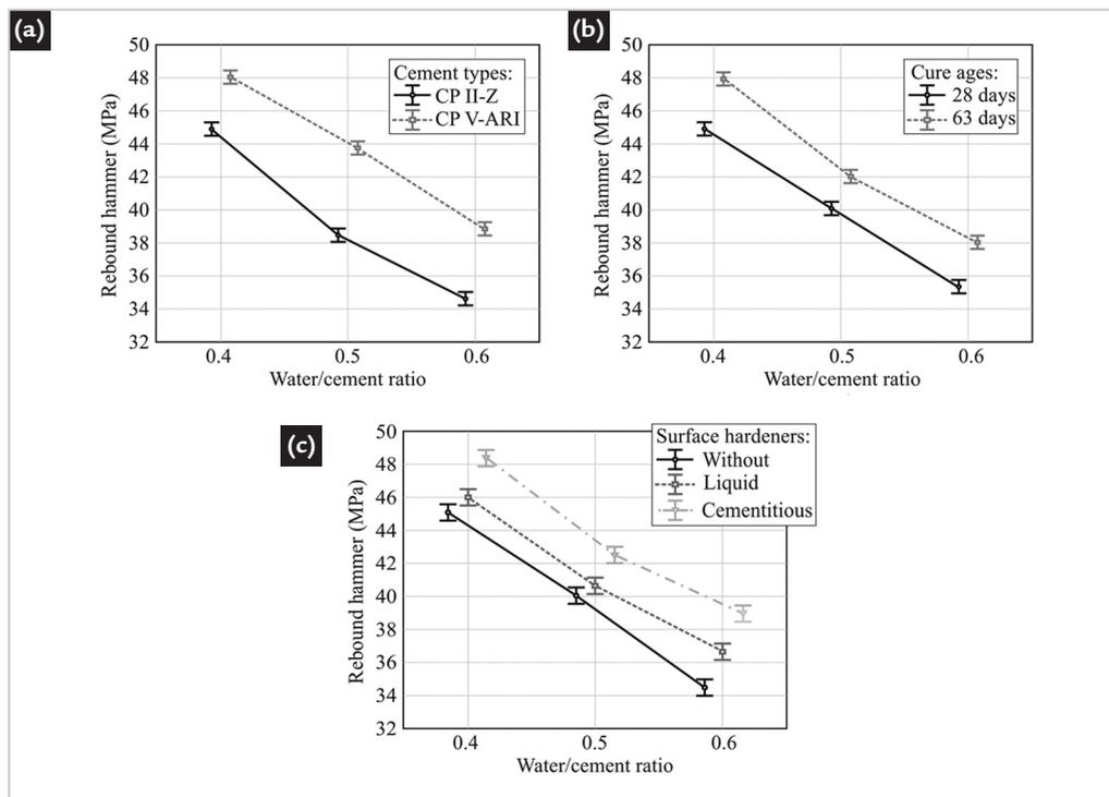
Figure 5 - Effects between the cement type and treatment type on the surface hardness.
