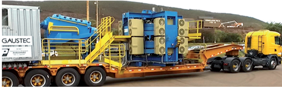
Figure 1 From the left side: Electrical Cabinet, NoBLOCK® Filter and GX-300 Super- WHIMS®.
