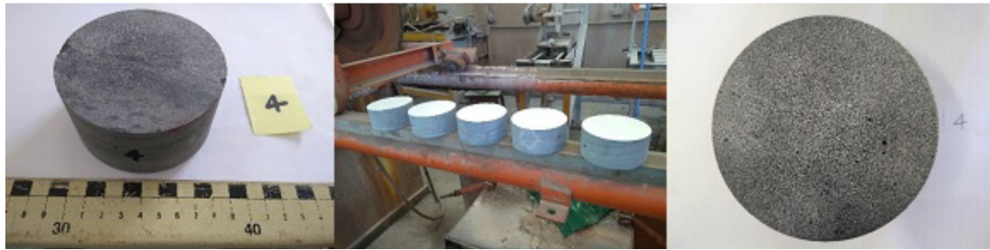
Figure 3 - Preparation of the specimen surface.
