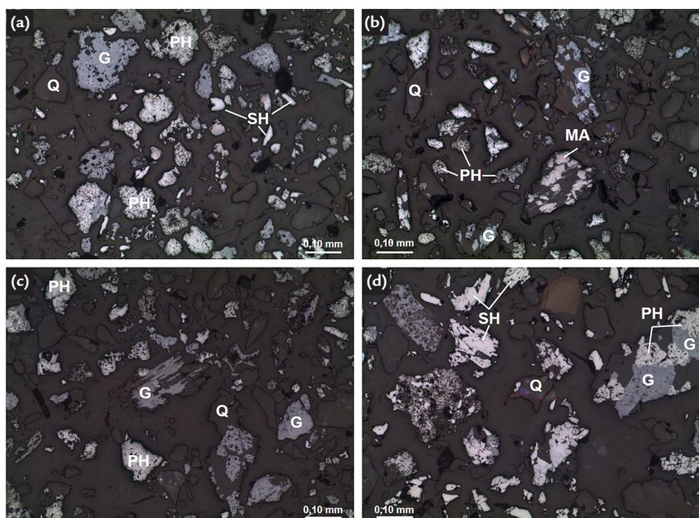
Figure 3 - Optical microscopy photos showing the general aspect of the ROM desliming samples. (a): AGEO 1; (b) AGEO 2; (c) AGEO 3 and (d) AGEO 4. SH - specular hematite; HP - porous hematite; G - goethite; Ma - magnetite; Q - quartz.
