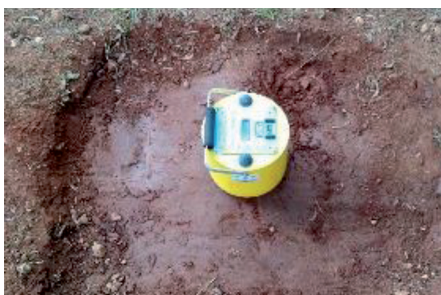
Figure 4 Test with the rigidity meter of compacted soils.
