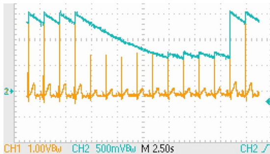
Figure 3. Simulated ECG (0.05-150Hz) and the output of the peak detector sampled by a dual channel oscilloscope (Tektronix – TDS2002C). As the rectifier circuit halves the amplitude of the ECG, the voltage scale of the channel 1 is twice (in terms of volts per division) that of the channel 2 to allow the superposition of the two curves. After few cycles, the simulated ECG amplitude was halved; the voltage across the capacitor of the peak detector drops exponentially until it reaches the new peak value.
