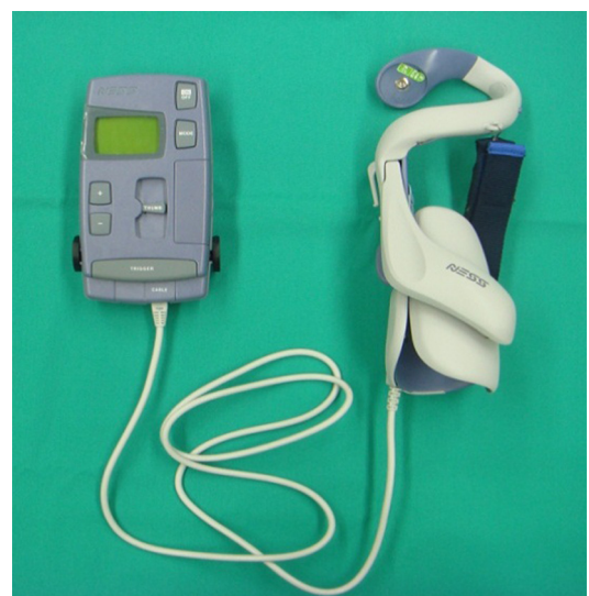
Figure 1. Handness® System. Right: the manually adjustable handle with five built-in electrodes to activate the index finger and thumb. Left: system control unit. Extracted from Shibata et al. (2013).
