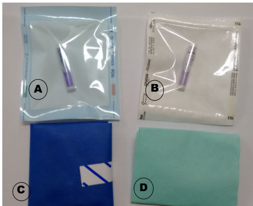
Figure 3. Pictures of the packaging studied. (A) = paper-plastic; (B) = Tyvec-plastic; (C) = SMS; and (D) = crepe paper. Inside each packaging, there is a self-contained ampoule with a biological indicator.
