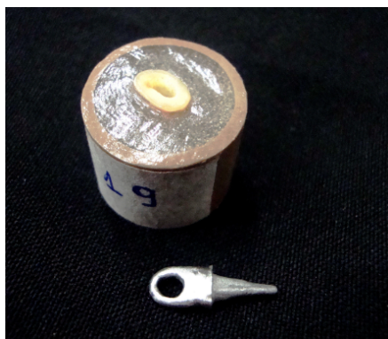
Figure 1. Casting cobalt-chrome alloy.
