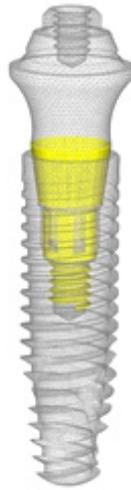
**Figure 3.** Regions of contact between implant, abutment and screw.
