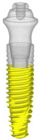
**Figure 4.** Region of fixation of implant-abutment system.
