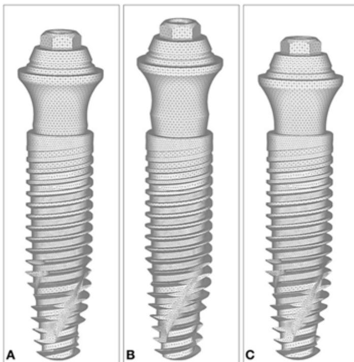
**Figure 2.** Three-dimensional tetrahedron mesh. A) (G1); B) (G2); and C) (G3).
