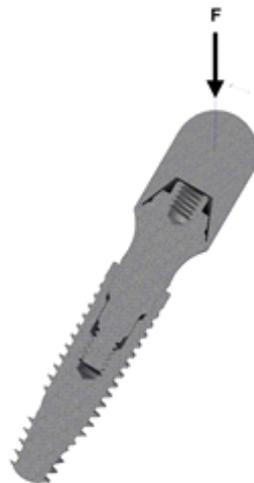
**Figure 5.** Schematic image showing the simulation test using a decentralized vertical load applied to samples, inclined 30 degrees to the vertical axis.
