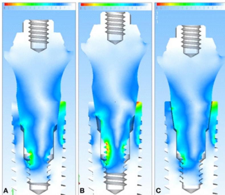
**Figure 6.** Finite element analysis results of stress behavior for the 32-N.cm torque under a 210 N load. A) G1; B) G2; C) G3. Red areas represent high stress regions, and as stress decreases, colors change to green and blue.
