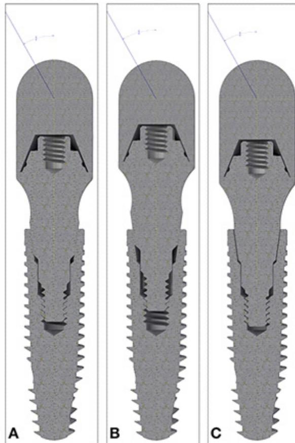
**Figure 1.** Study Groups. A) G1: GM Mini Conical Abutment with cone diameter dimensions as recommended by the manufacturer ( $\varnothing 3.11$  mm); B) G2: GM Mini Conical Abutment with cone diameter 6.1% larger than G1 Abutment ( $\varnothing 3.3$  mm); C) G3: GM Mini Conical Abutment with cone diameter 6.1% smaller than G1 Abutment. ( $\varnothing 2.92$  mm). All abutments were 3.5-mm high and all assemblies had 4.0x13 mm Helix GM implants.
