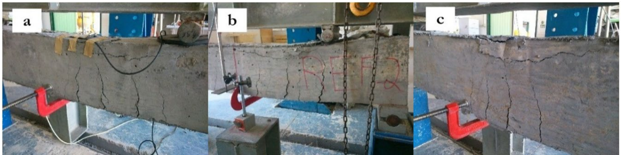
Figure 10. Beams of the reference group (REF) after four-point bending tests a) REF-1. b) REF-2. c) REF-3.
