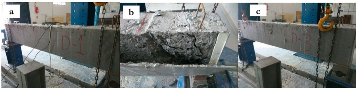
Figure 11. Beams of the group D after four-point bending tests. a) D-1. b) D-2. c) D-3.
