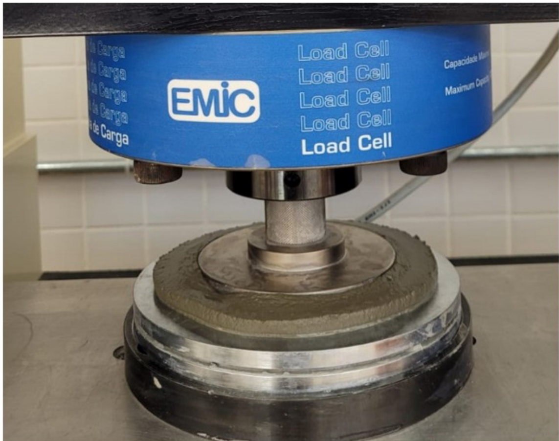
Figure 4. Illustration of the squeeze-flow configuration
