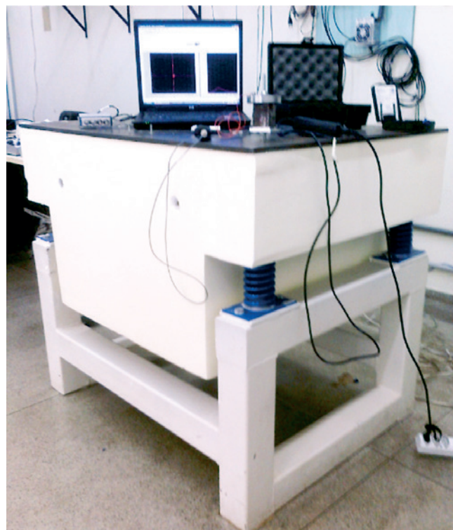
Figure 6 Inertial table with experimental apparatus for AME realization
