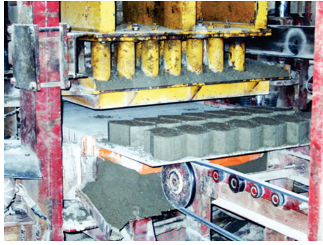
Figure 5 – Vibropress used in the production of the concrete blocks
