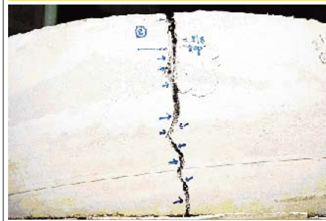
Figure 18 - Cracked ring after the test
