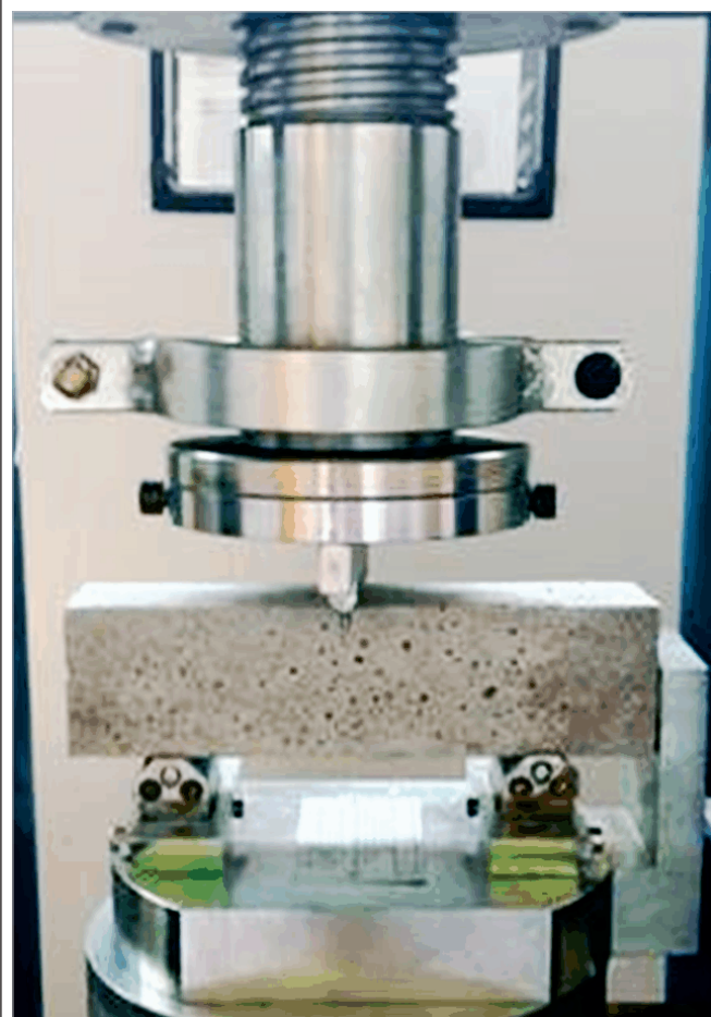
Figure 9 – Testing of prismatic mortar specimen by simple flexion and by compression
