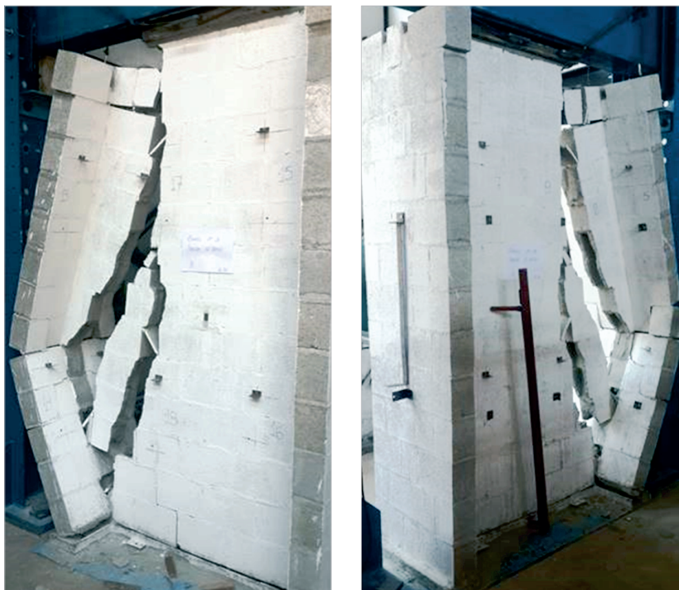
Figure 17 - Failure - flanged wall without central support 06
