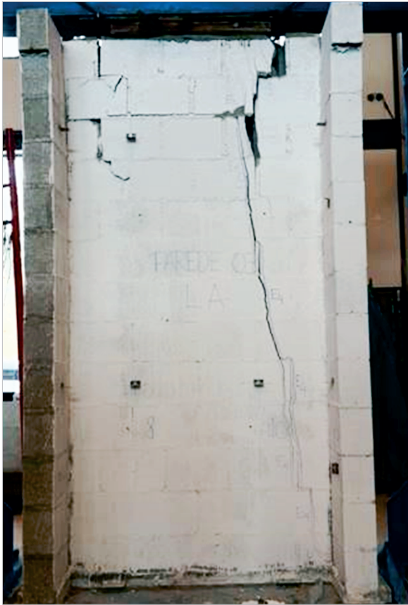
Figure 14 - Failure - flanged wall with central support 03
