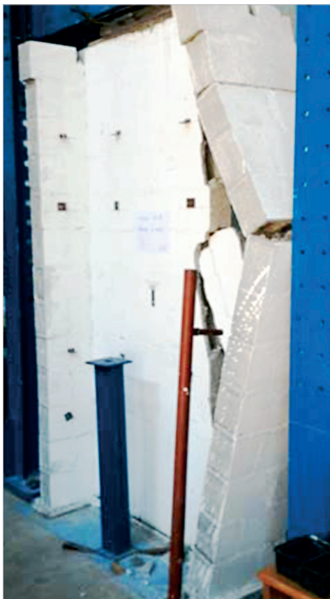
Figure 15 - Failure - flanged wall without central support 04
