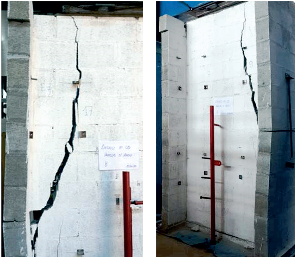
Figure 16 - Failure - flanged wall without central support 05
