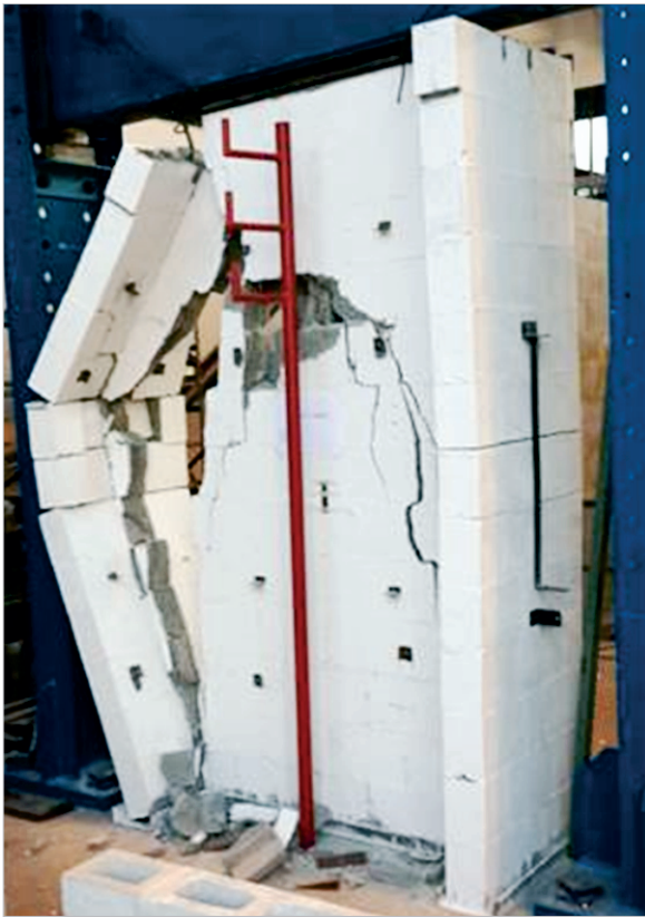
Figure 12 - Failure - flanged wall with central support 01
