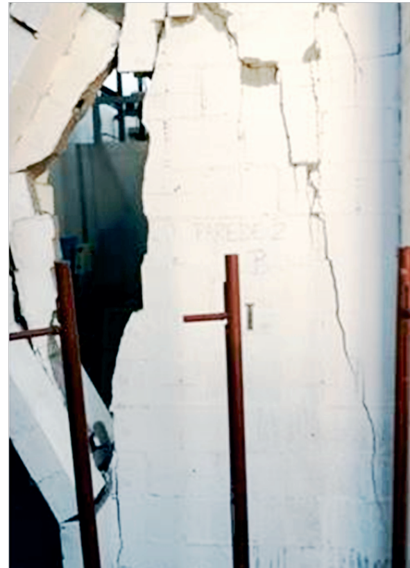
Figure 13 - Failure - flanged wall with central support 02
