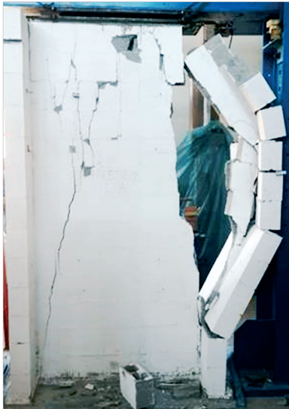
Figure 13 - Failure - flanged wall with central support 02
