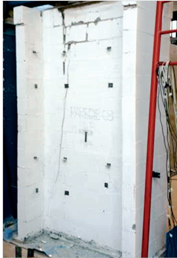
Figure 14 - Failure - flanged wall with central support 03
