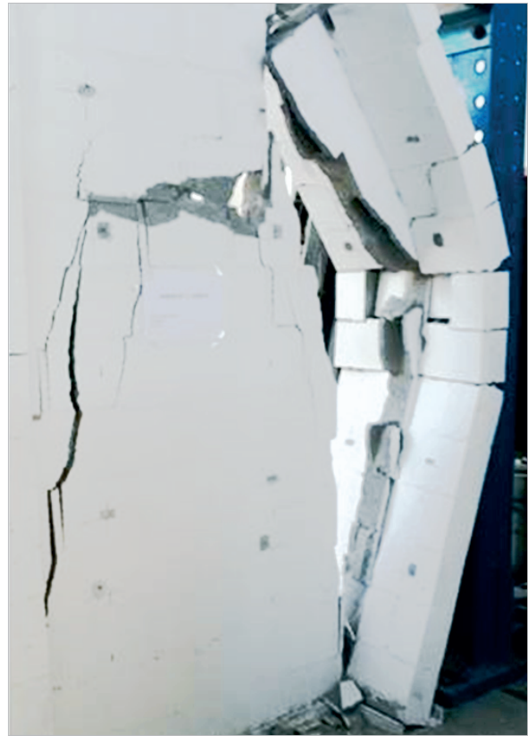
Figure 12 - Failure - flanged wall with central support 01
