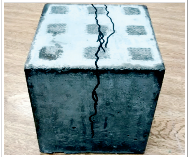
Figure 7 - Cracks formation in compressive stresses transfer test in blocks containing protuberances in the connected surface
