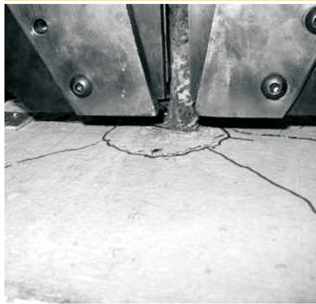
Figure 10 – Shear cone originated from reinforcement steel pull out process
