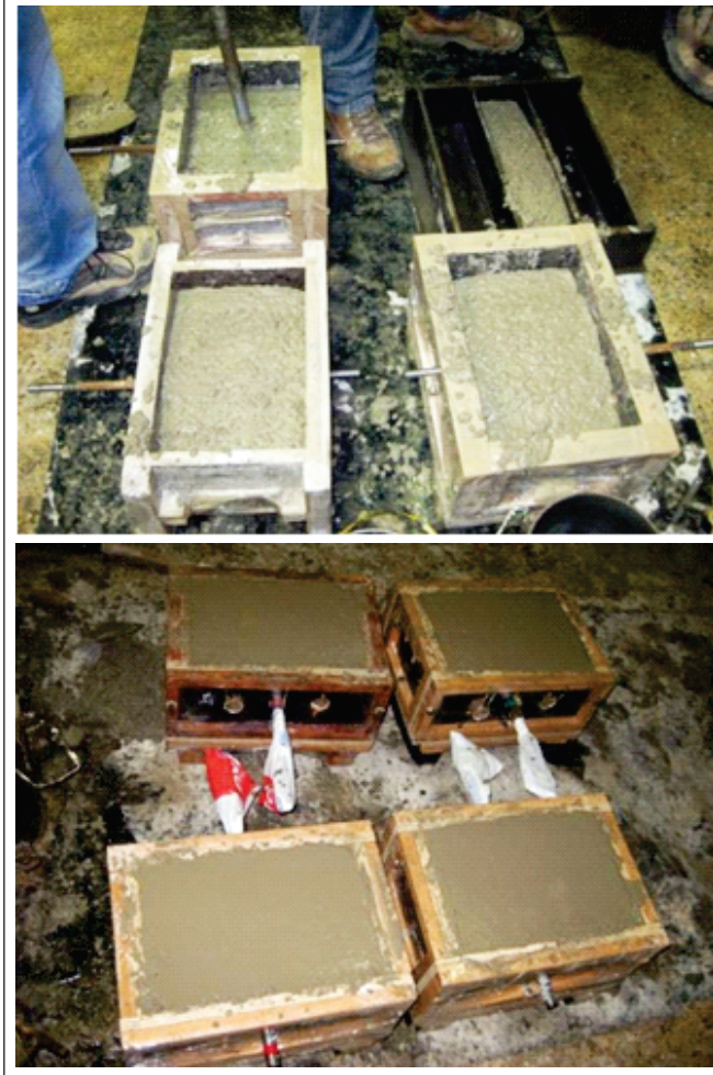
Figure 2 – Molding of test specimens for the pull-out test
