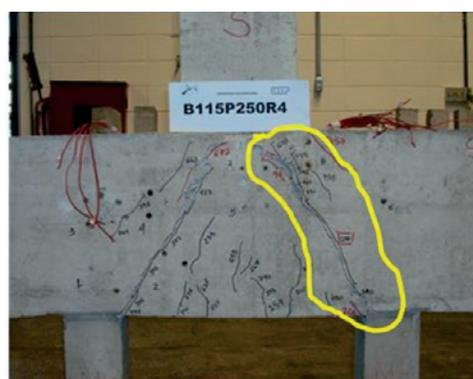
Opening inclined cracks (failure models)
