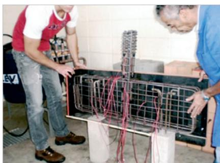
Installation of reinforcement pile caps in molds
