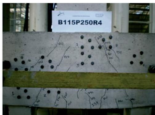
Propagation inclined cracks
