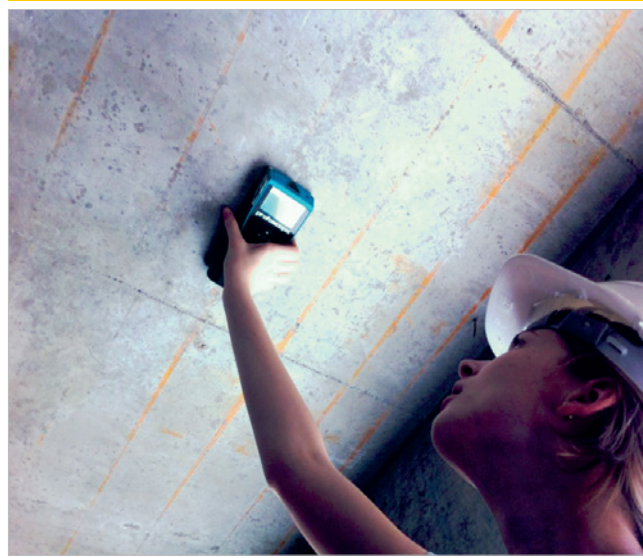
Figure 10 – Measuring the cover of the positive reinforcement of the slabs
