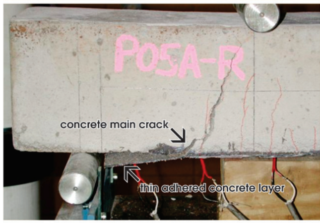
Figure 1 - Strengthened beam failure by debonding (Ferrari (1))
