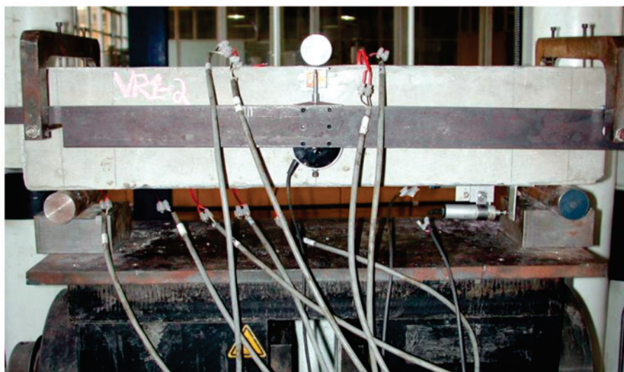
b) General aspect of flexural test in three points
