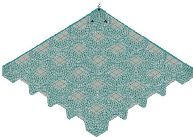
Figure 9 Finite element mesh for the VL3A model with 22,278 finite elements
