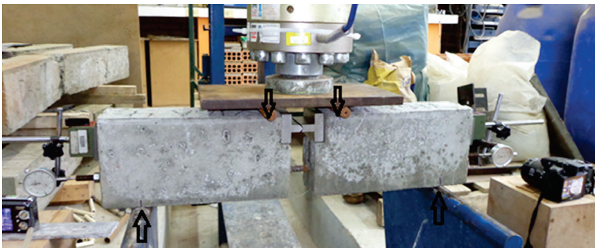
Figure 3 - Execution of the beam test
