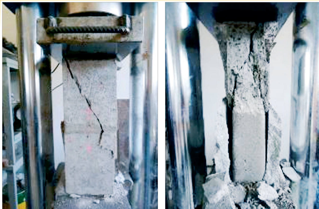
Figure 22 Hollow and grouted prism testing
