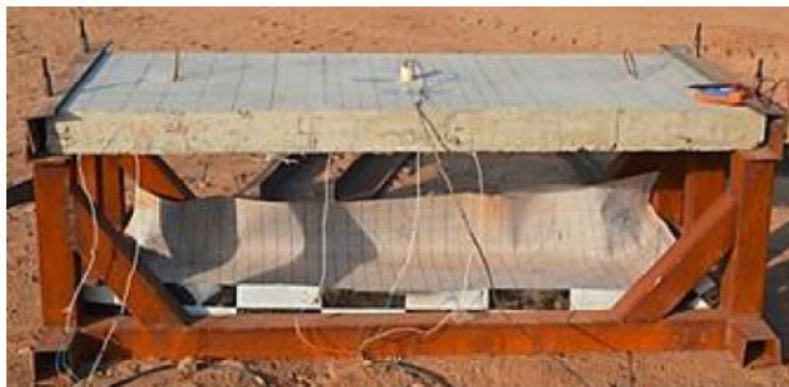
Figure 3 - Test setup of the slab specimens tested by Li et al. [10]
