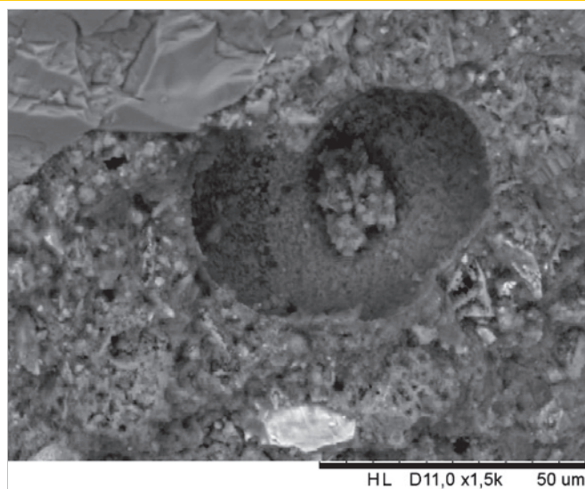
Figure 6 – Microscopy of mortar specimens with 30% replacement by steel slag (800x, 1500x, and 2500x)
