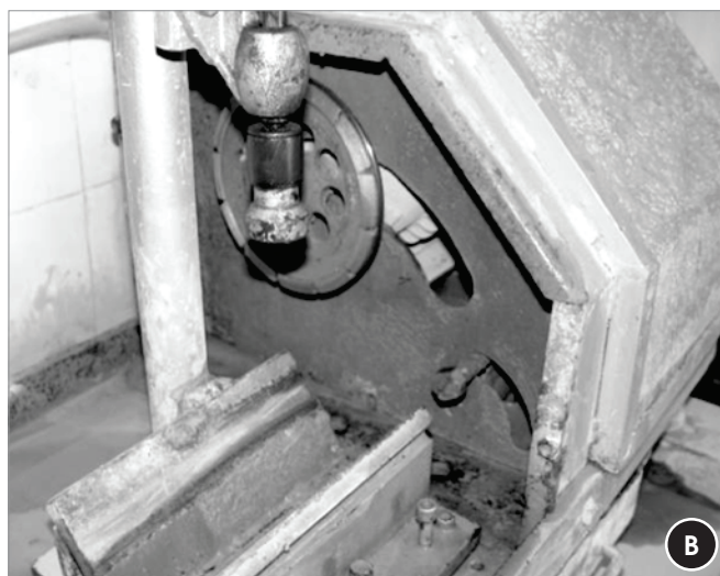
Figure 2 – Test specimen grinding in RRDF grinder (B) and flexible diamond wheel (A)
