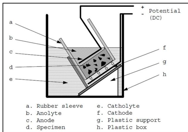
Figure 6. Arrangement of the migration set-up. Source: Nordtest [2]
