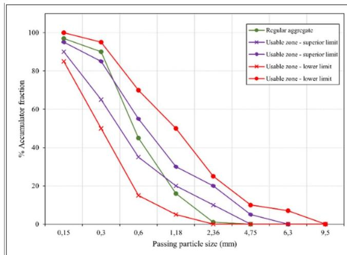
**Figure 1.** Granulometric curve of the natural fine aggregate
