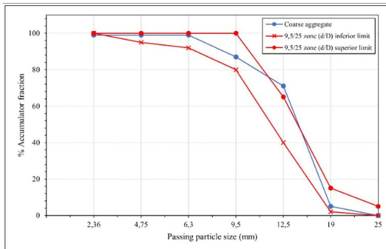
**Figure 5.** Granulometric curve of the coarse aggregate
