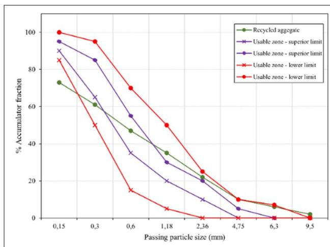
**Figure 3.** Granulometric curve of the recycled fine aggregate.
