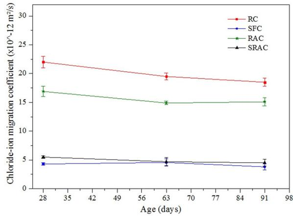
Figure 10. Graph of average chloride ion penetration coefficient.
