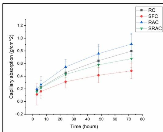
**Figure 9.** Results of capillary water absorption at different exposure periods.
