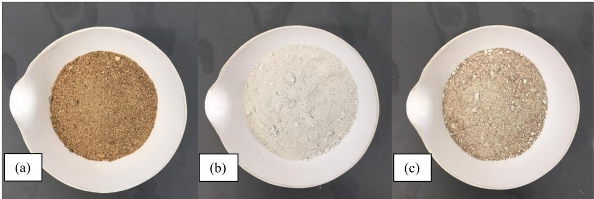
**Figure 4.** Aspect of the materials used as fine aggregates. a) natural fine aggregate; b) recycled fine aggregate; c) fine aggregate with 30% of replacement of fine natural aggregates by recycled fine aggregates
