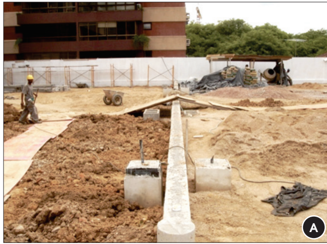
Figure 7 – (a) Unevenly distribution of the load and (b) Slab totally loaded
