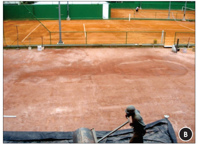
Figure 7 – (a) Unevenly distribution of the load and (b) Slab totally loaded
