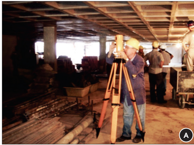
Figure 5 – Vertical displacements measurement
