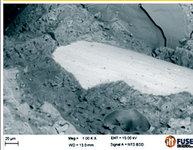
Figure 9 – SEM image of steel fiber interface with the cementitious composite
