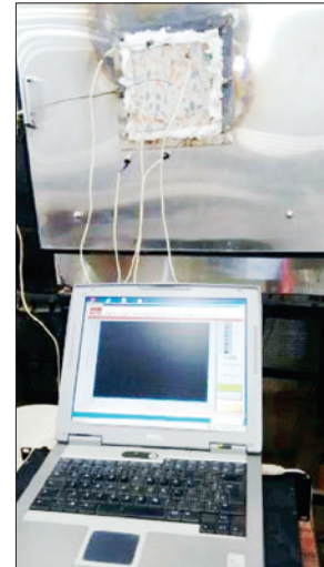
Figure 1b Sample positioned for the evaluation of spalling
