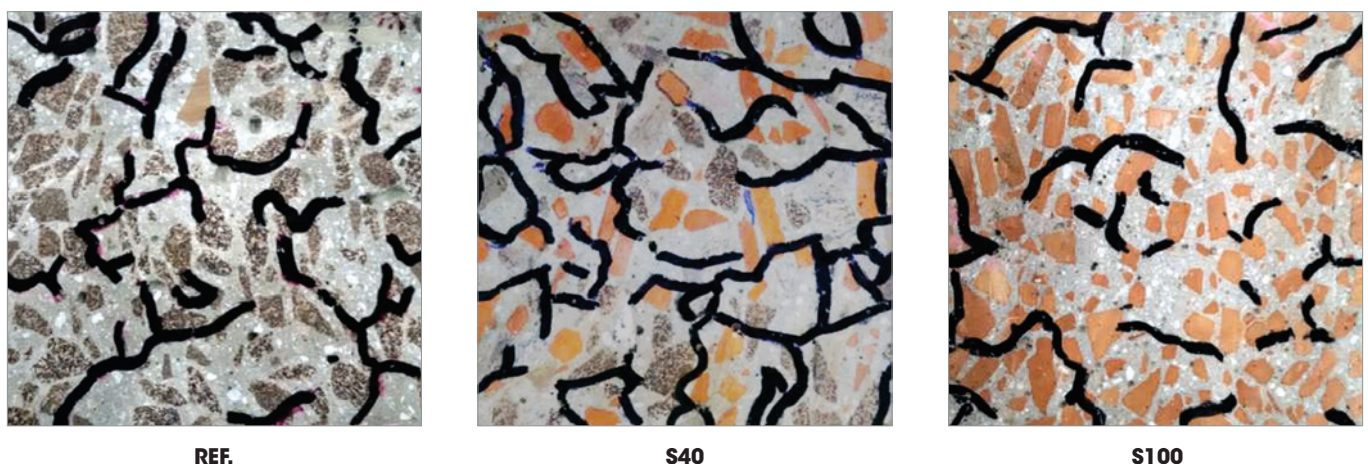
Figure 4 Specimens after the evaluation of explosive spalling (temperature: 925°C)
