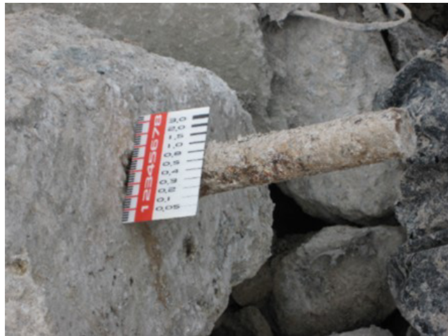
Figure 5. Concrete block with dowel at the crushing plant.
