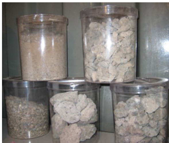
Figure 6. Different particle size fractions obtained following primary jaw crushing.
