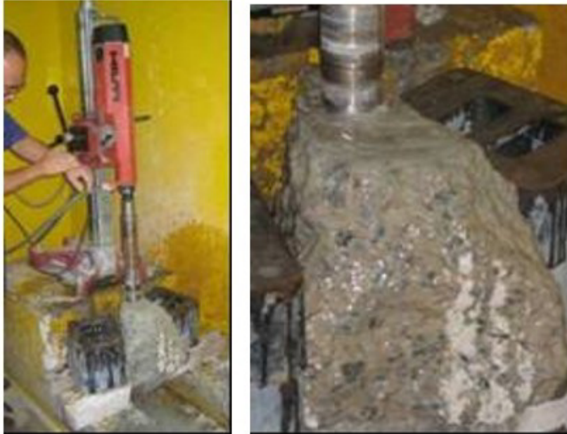
Figure 7. Extraction of cylindrical cores from the original pavement blocks.
