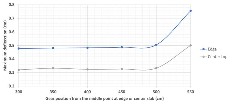
Figure 8. Maximum deflections caused by main gear A 320-200 on concrete.
