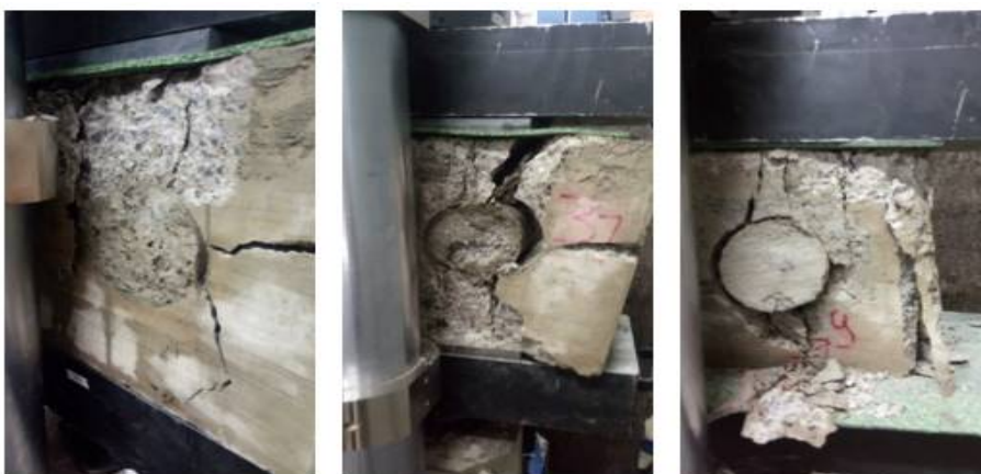
Figure 8 – Fracture characteristics of each repaired block (left to right: C20, grout and dry pack)
