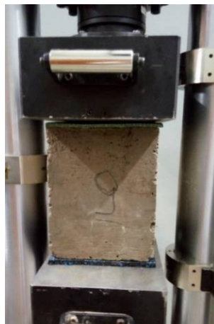
Figure 5 – Compression test in universal press
