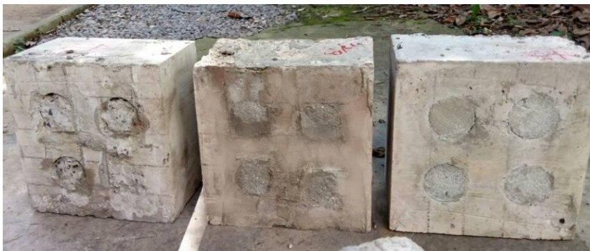
Figure 4 – Finalized repaired blocks with concrete, grout and dry pack (left to right)
