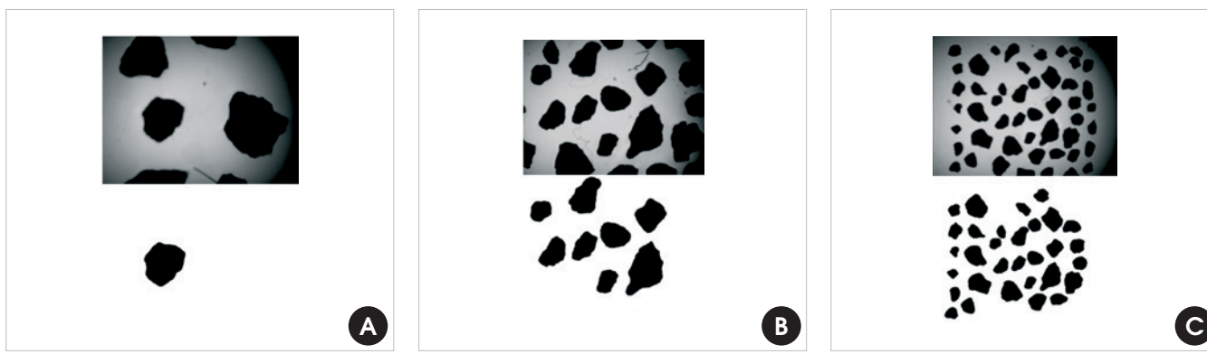
Figure 3 – Zoom effect used for the obtention of the images of the grains: (a) 3.0X, before and after treatment, (b) 1.5X, before and after treatment and (c) 0.7X, before and after treatment
