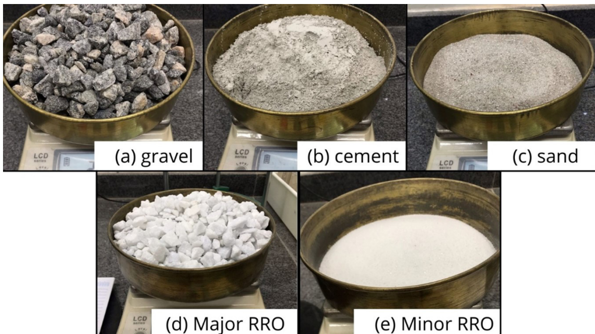
Figure 1. Materials used in the mass to produce concrete: (a) gravel; (b) cement; (c) sand; (d) Major RRO and (d) Minor RRO.
