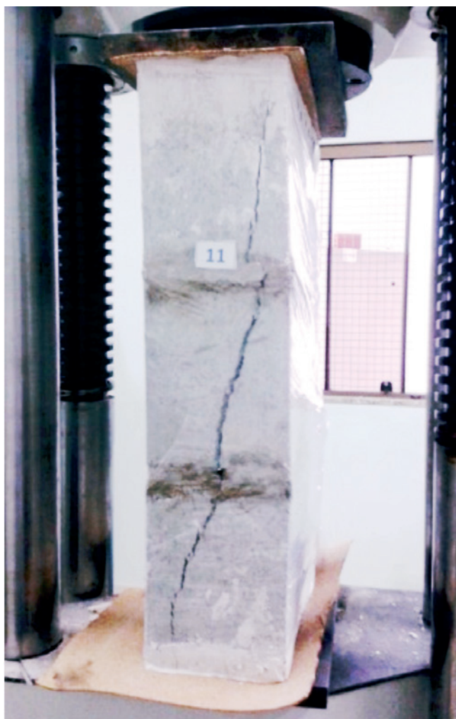
Figure 6 Axial compression trial of three block laid prisms
