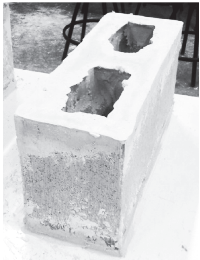
Figure 2 Block with plaster capping
