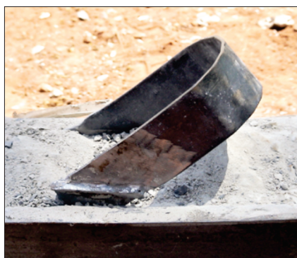
(b) Arc-shaped connector Q_{Rm} = 180.0 \text{ kN} (Chaves[2])
