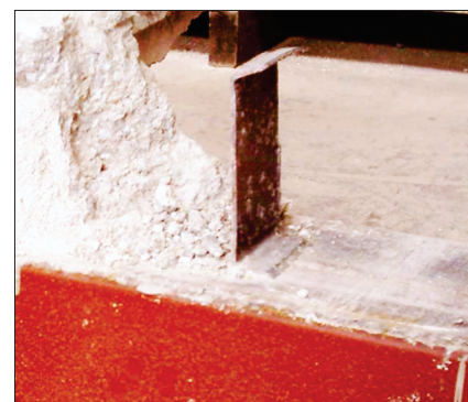
(c) Channel connector 120x25x3 Q_{Rm} = 245.1 \text{ kN} (Bremer[3])
