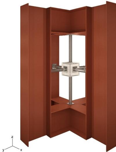
**Figure 1** -Simplified illustration of Liaudat et al. [23] ‘alkali-aggregate reaction triaxial machine’.
