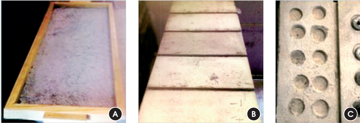
Figure 1 – (a) Standard concrete substrate and mold for mortar application, (b) cure of the mortars applied for standard substrate and (c) mortar after adhesion test
