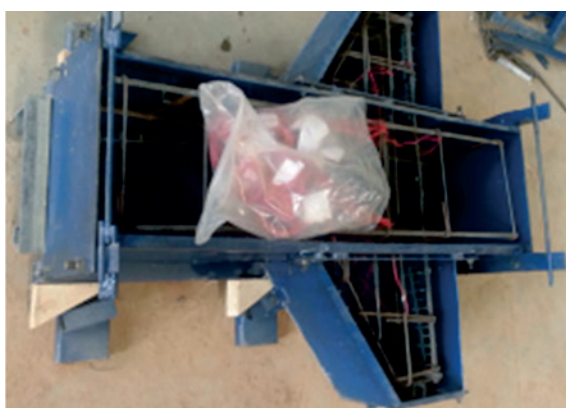
(a) Formwork for cast monolithic model
