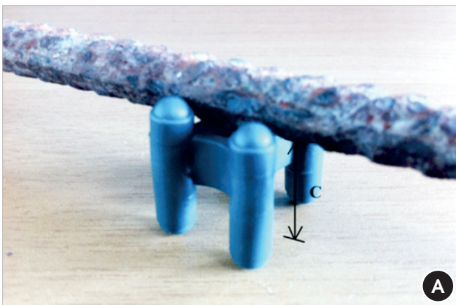
Figure 7 – Evaluation method of the design requirement: a) in chair-type spacers; b) in circular spacers
