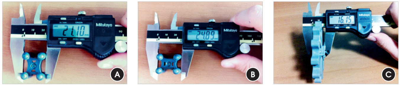
Figure 8 – Measurement of the dimensions of chair-type spacers: a) measured parallel to the bar position; b) measured perpendicular to the bar position; c) measured from center of support of the circular spacer
