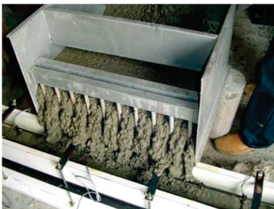
Figure 9 – a) Casting of the SCC beam; b) Compacting of beams in the vibrating table (RC and SFRRC)
