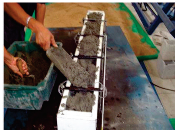
Figure 9 – a) Casting of the SCC beam; b) Compacting of beams in the vibrating table (RC and SFRRC)
