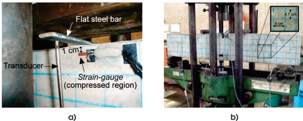
Figure 11 – Bending test for the reinforced concrete beam: a) Detail of the strain-gauge placement in the region of compressed concrete and b) Rectangular mesh for the mapping of cracks
