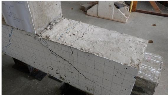
Figure 9. BEmb20sch failure plans.
