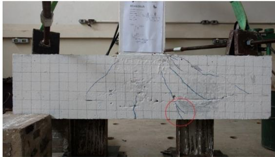
Figure 8. Failure plane of the BEmb10cch model.
