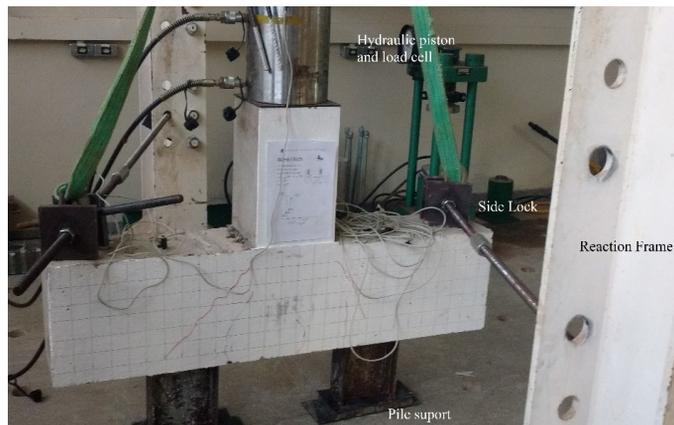
Figure 6. Test-system configuration.
