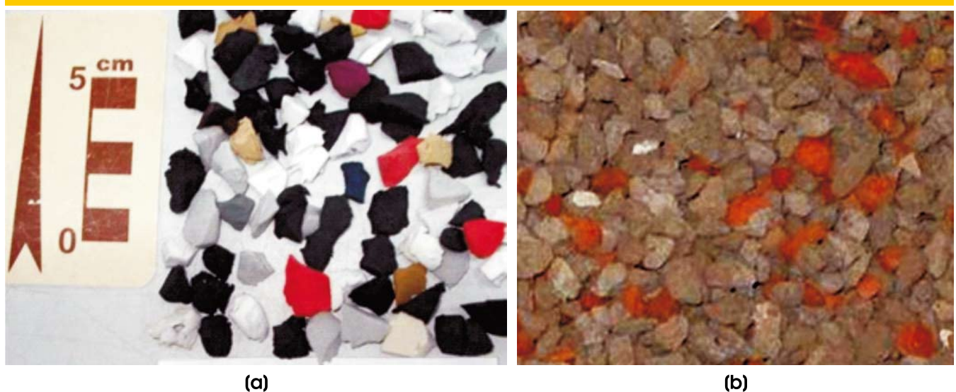
Figure 2 – Recycled coarse aggregates used in this research: a) EVA; b) RCA
