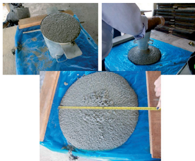
Figure 1 Slump flow test of SLCEB From: Catoia (2), p. 55
