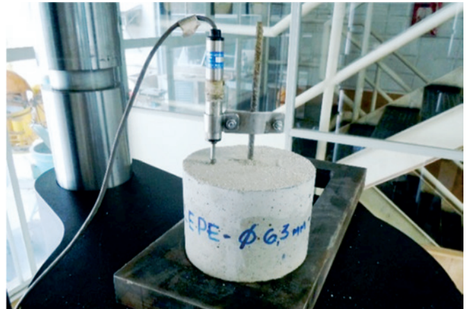
Figure 10 Position of inductive transducer of displacement
